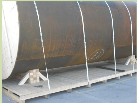
Figure 6 - Saddles for stacks, silencers etc.
